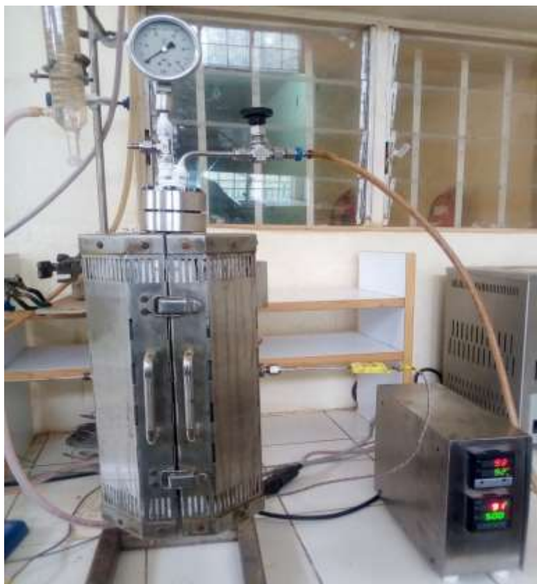
Plate 2.2: Set up for Hydrodeoxygenation of Furfural-Acetone adduct to Hydrocarbon fuels
