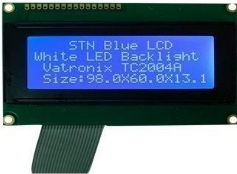
Figure 3. 8 4-line 20-character alphanumeric LCD
