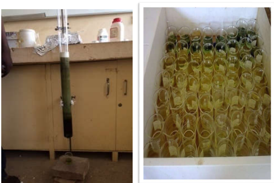
Figure 4.8: Silica-gel Column Chromatography and Eluted Fractions from Chromatographic Purification of Methanol fraction..
