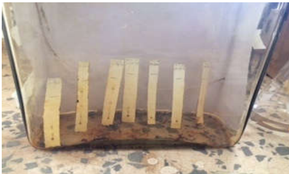
Figure4.7: TLC Analysis of the Crude Methanol fraction F4 of Moringa oleifera Viewed inside Iodine Chamber showing Spots of Different Compounds
