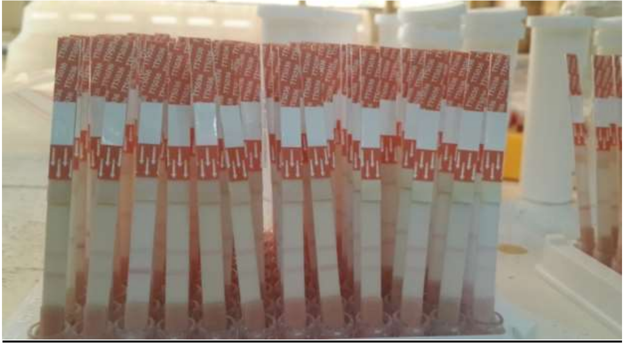
Plate 3: Dipsticks Inserted into Reagent Vials and Incubated at Room Temperature
