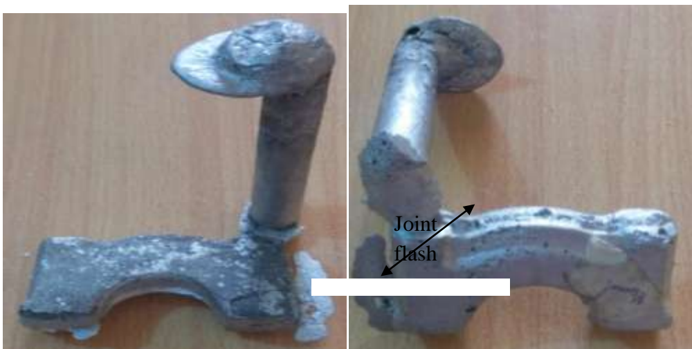
Plate 4.11: Cope side of the bearing cap cast using hand-shank ladle pouring Plate 4.12: Drag side of the bearing cap cast using hand-shank ladle pouring
