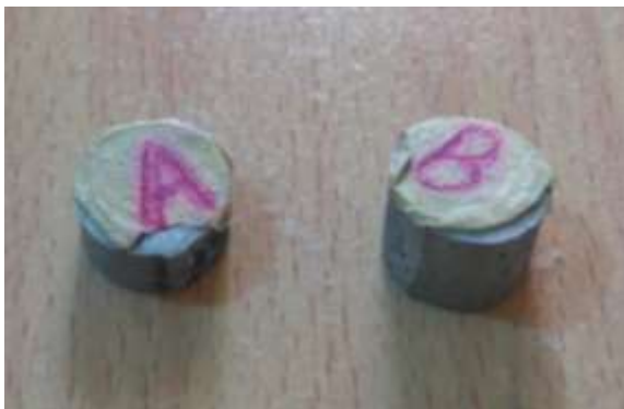
Plate 3.5: Samples for metallography test. Where sample A was from pouring ladle and sample B from hand-shank ladle
