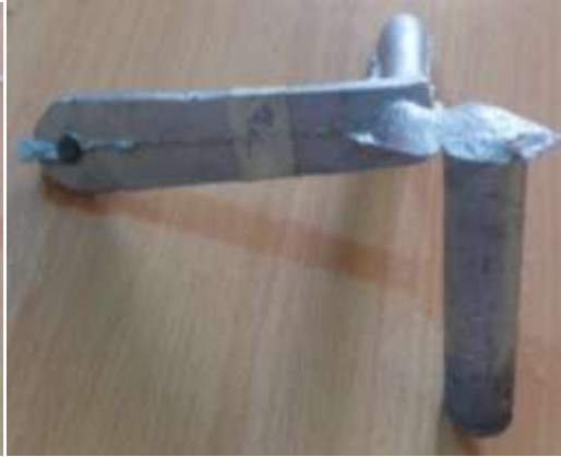
Plate 4.4: Rear side of the crank lever cast using ladle machine pouring
