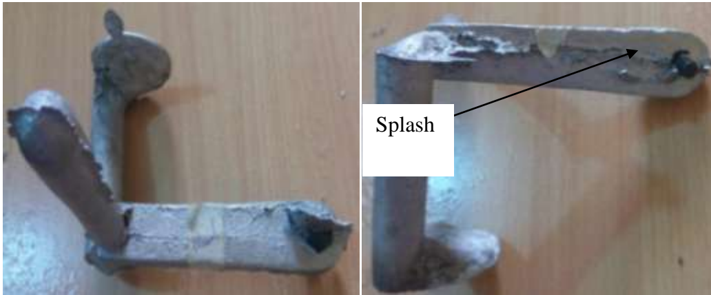
Plate 4.9: Front side of the crank lever cast using hand-shank ladle pouring Plate 4.10: Rear side of the crank lever cast using hand-shank ladle pouring
