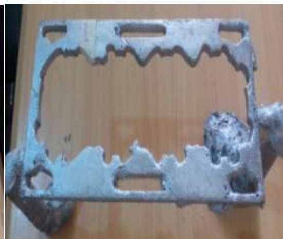
Plate 4.8: Drag side of the water jacket cast using hand-shank ladle pouring
