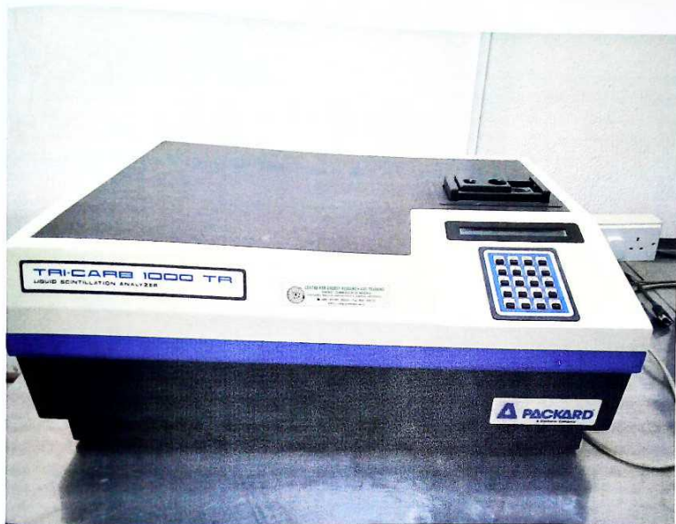
Figure 3.8 Liquid Scintillation Analyzer (Tri-carb- LSA 1000), Centre for Energy Research and Training (CERT), Ahmadu Bello University, Zaria.
