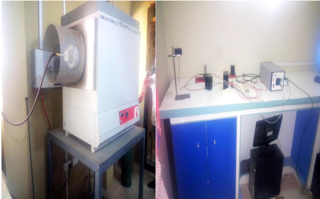
Figure 3.2(a) Carbolite tubular oven (b) Single beam spectrophotometer Avantes from MSE, KWASU.
