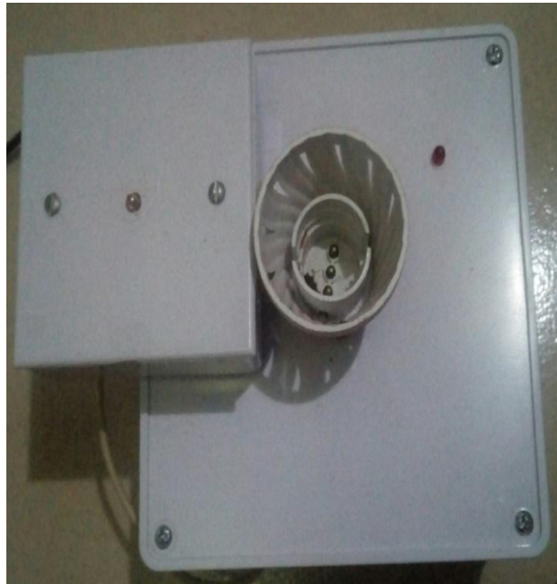
Figure 3.5: Casing and assembling of darkness activated switch
