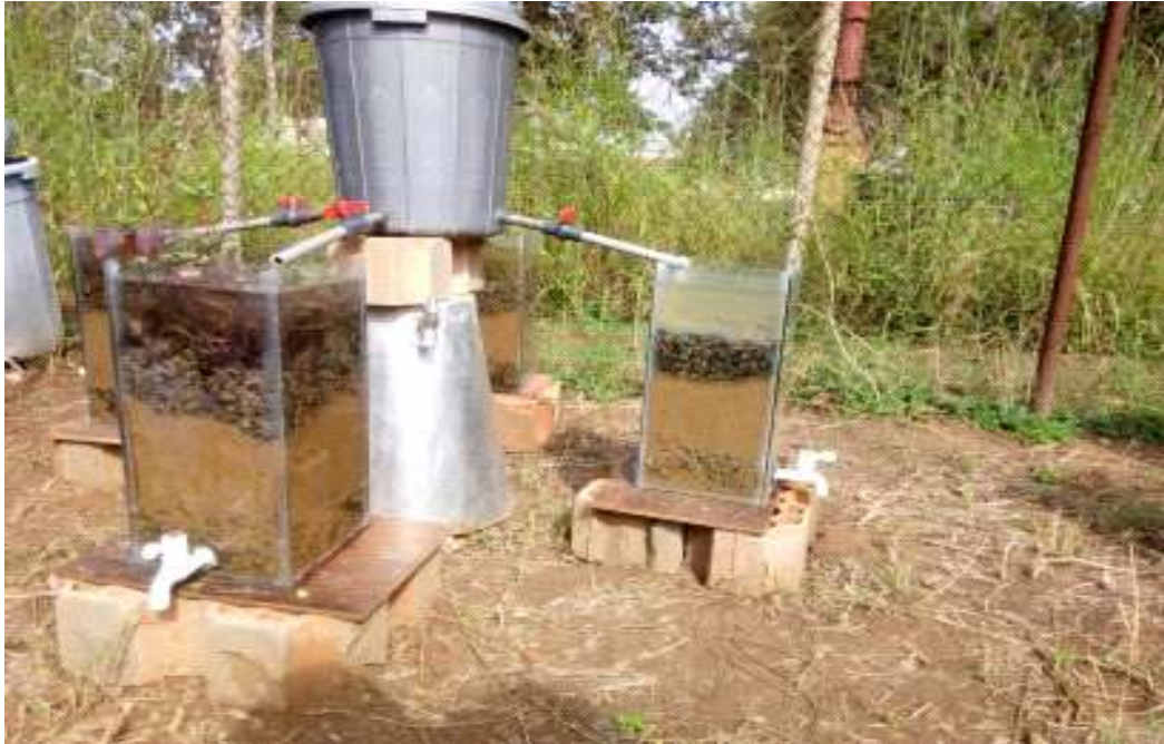
Plate XII: Batch flow experimental setup fully recharged with untreated sample.
