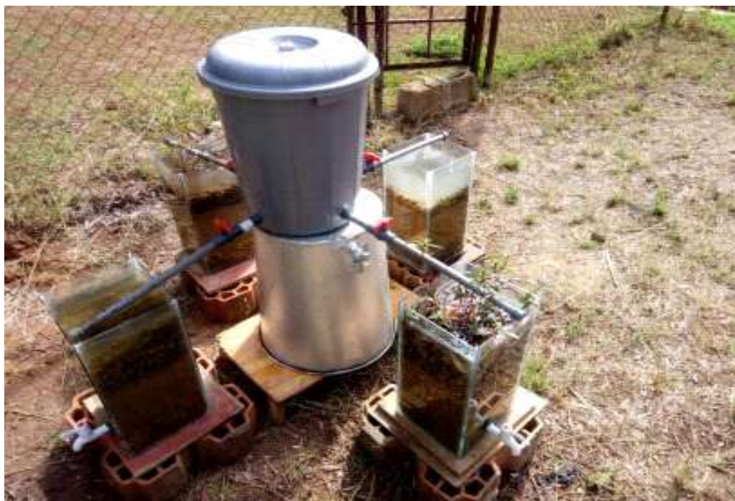
Plate XI: Continuous flow experimental setup fully recharged with untreated sample.
