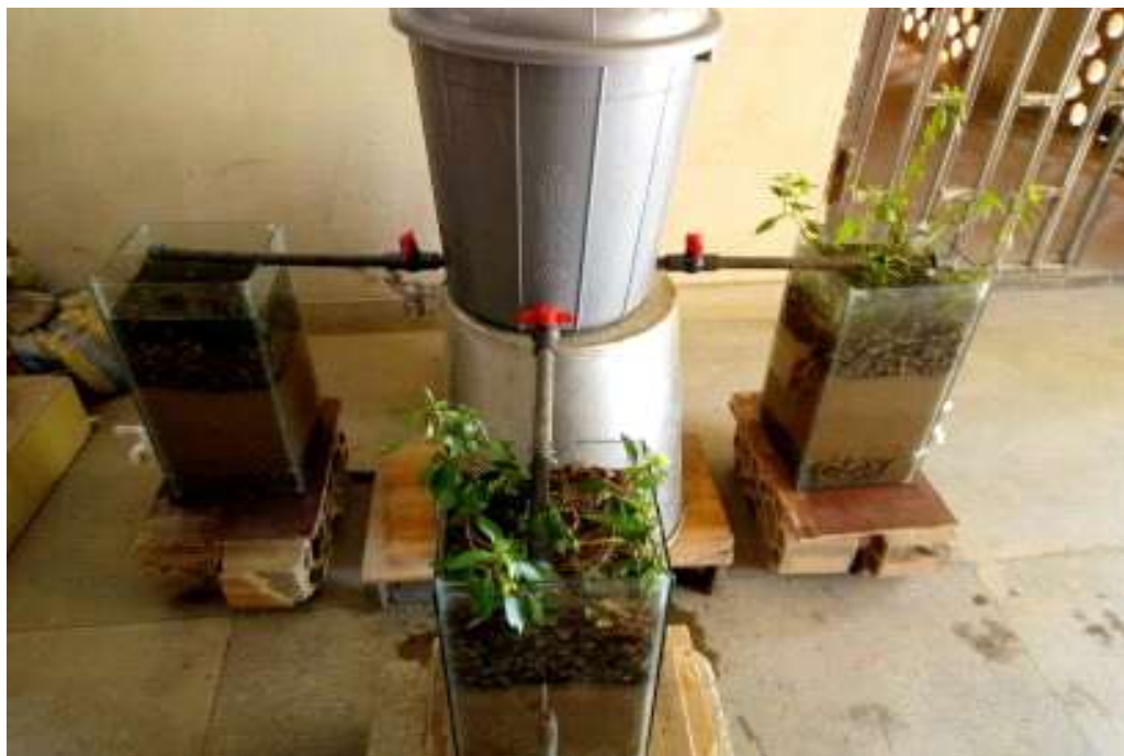
Plate XI: Continuous Flow: Experimental set-up showing the various plants moist with tap water prior to untreated effluent recharge.
