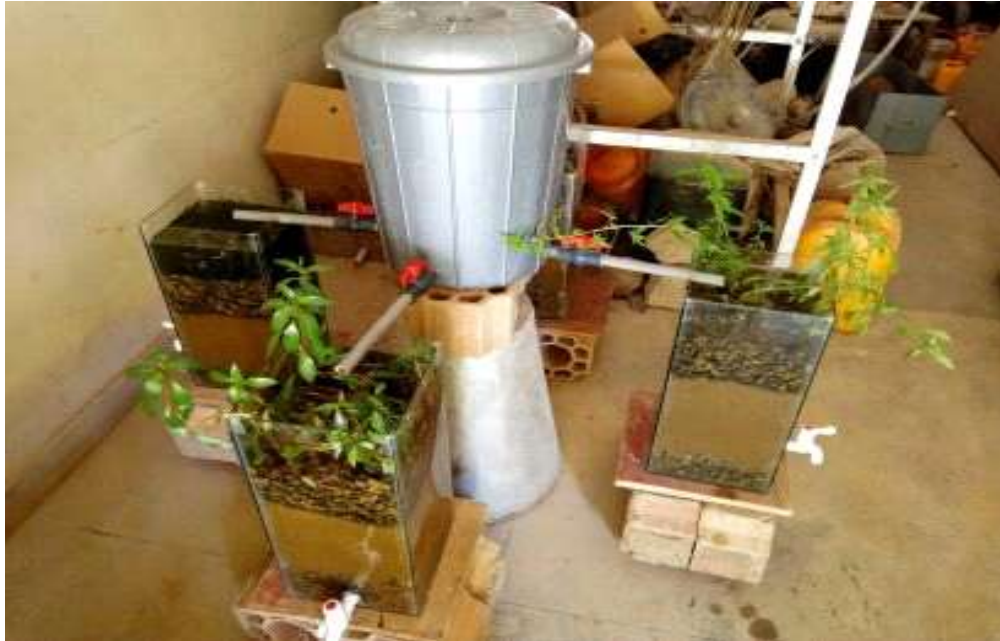
Plate X: Batch Flow: Experimental set-up showing the various plants moist with tap water prior to untreated effluent recharge.
