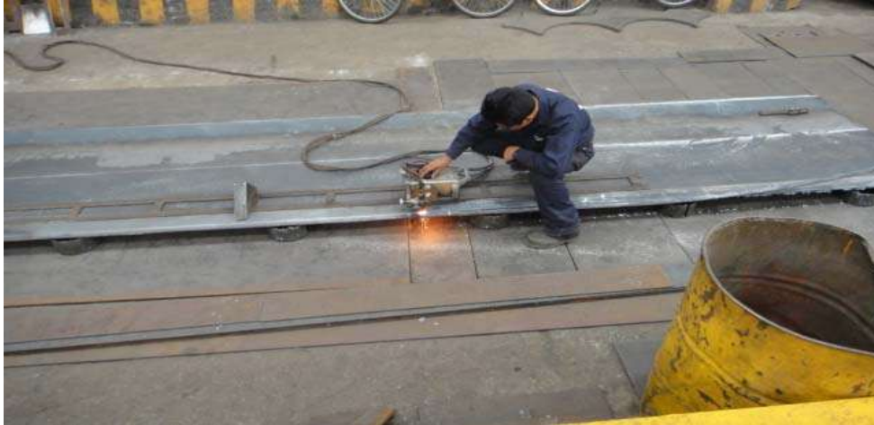
Plate I: Cutting of plate for poles(Edgar, 2016)
