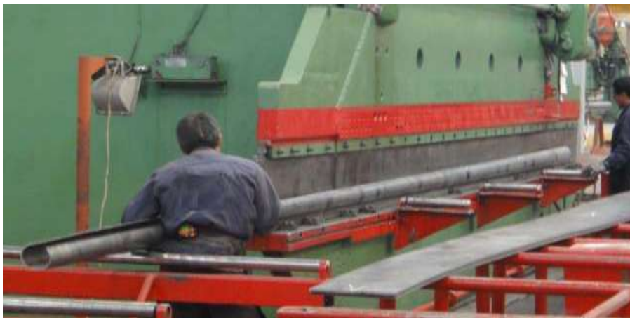
Plate II: Bending of the plate with hydraulic press
