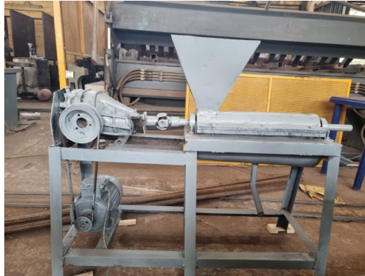
Fig. 3.2; Power Transmission of Coconut Oil Expeller
