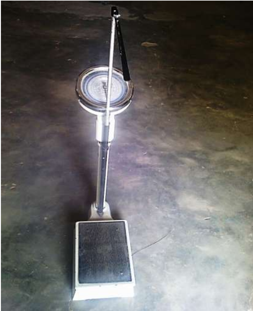
Plate I: A Stadiometer (Model RGZ 160, China) for measuring height and weight.
