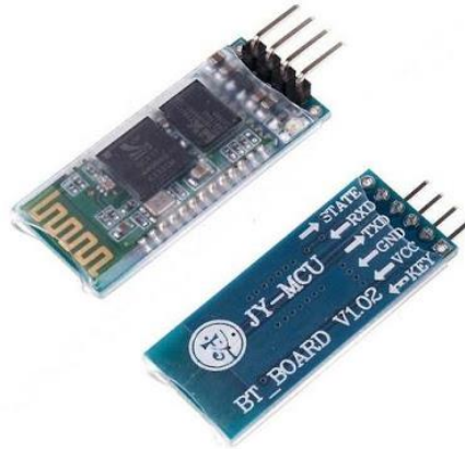
Figure 3.13: HC06 Bluetooth module
