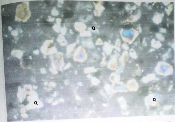
Fig.19 Photomicrograph of sample A under cross nicols showing poorly sorted sediments. Quartz is represented as (Q).
