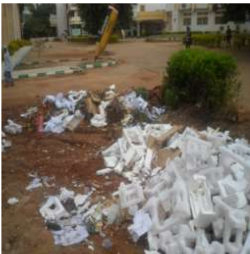
Plate III: A waste form of EPS
