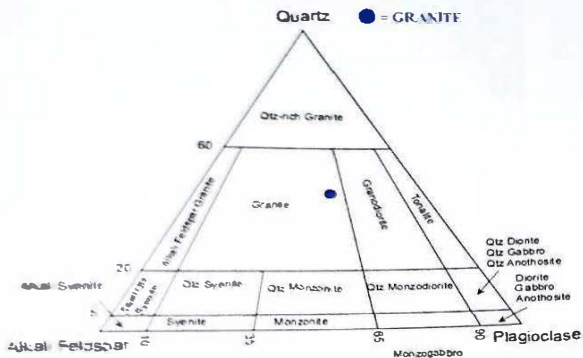
Fig 8: QAPF diagram of Sample A naming its composition as that of Granite.
