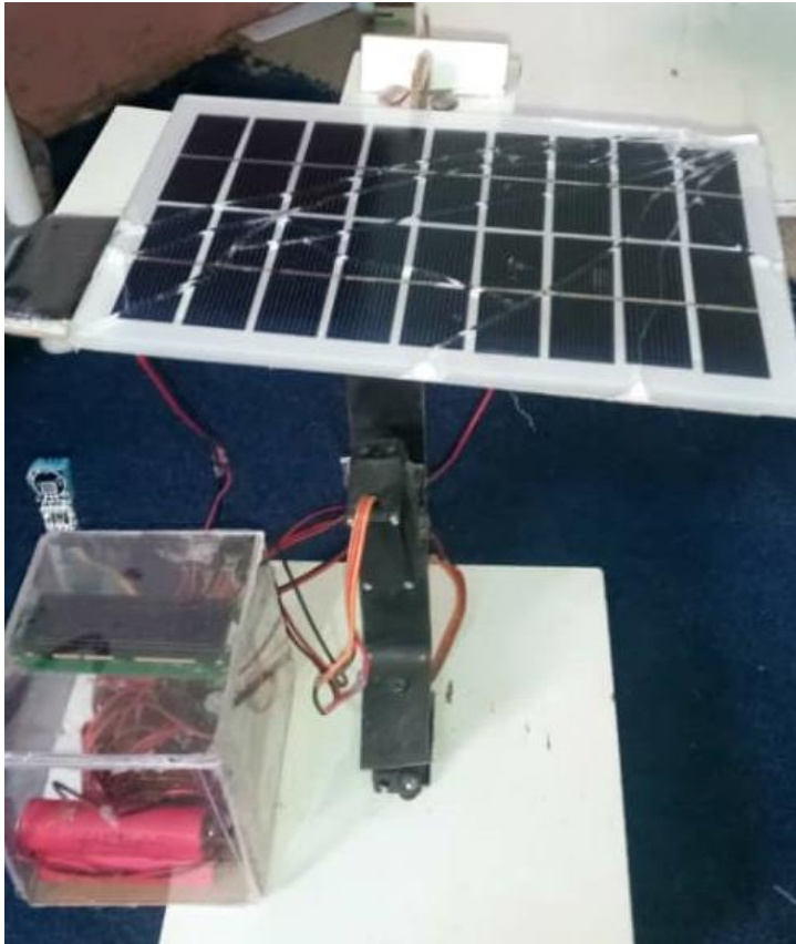
Plate 4.2 constructed solar tracking system
