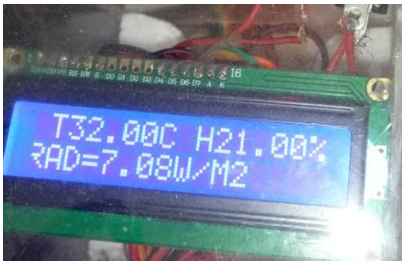
Plate 4.3 temperature, humidity and solar intensity display.
