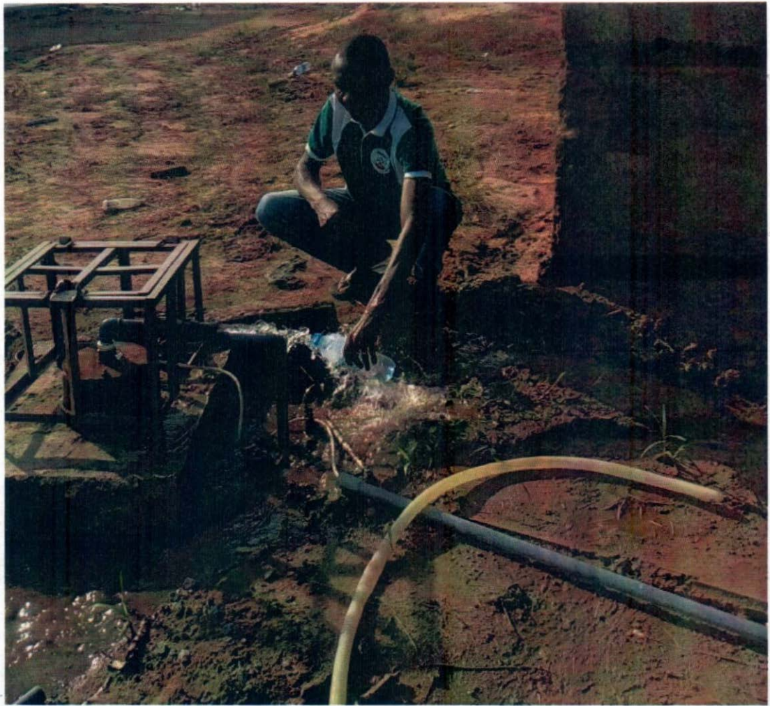
PLATE 4: Photograph showing purging and collection of representative sample from a borehole at location 6BH (N 5° 1' 54.0", E 8° 22' 2.4")
