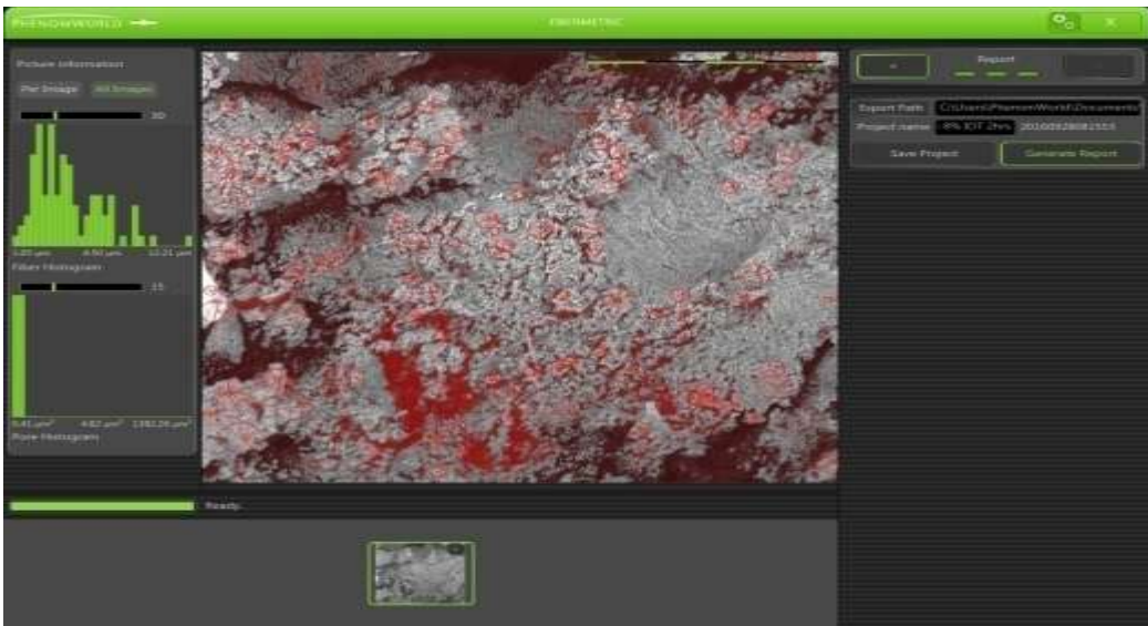
Plate 4.8: Fiber and pore image measurements of black cotton soil optimally stabilized with 8 % lime / 8 % iron ore tailings blend after 28 days curing period
