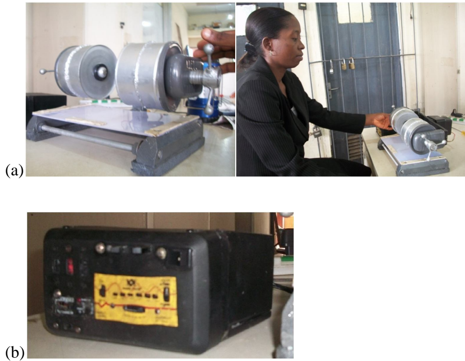
Fig.3.2 (a) Laboratory electromagnet, (b) current regulator
