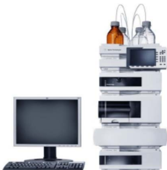
Modular HPLC System –high-end configuration with quaternary pump, autosampler, column thermostat, diode array detector, and computer with control and data analysis SW
