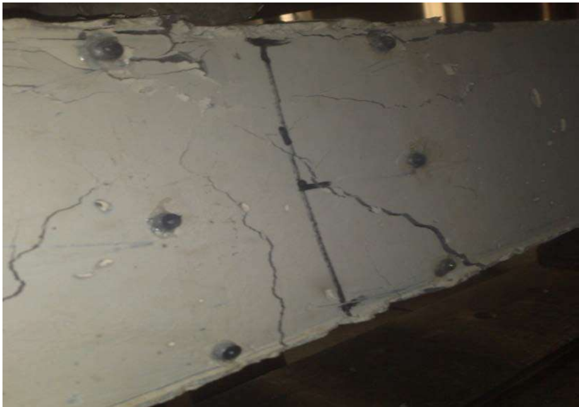
Plate 4.2: Crack pattern at critical section of beam at ultimate loading stage
