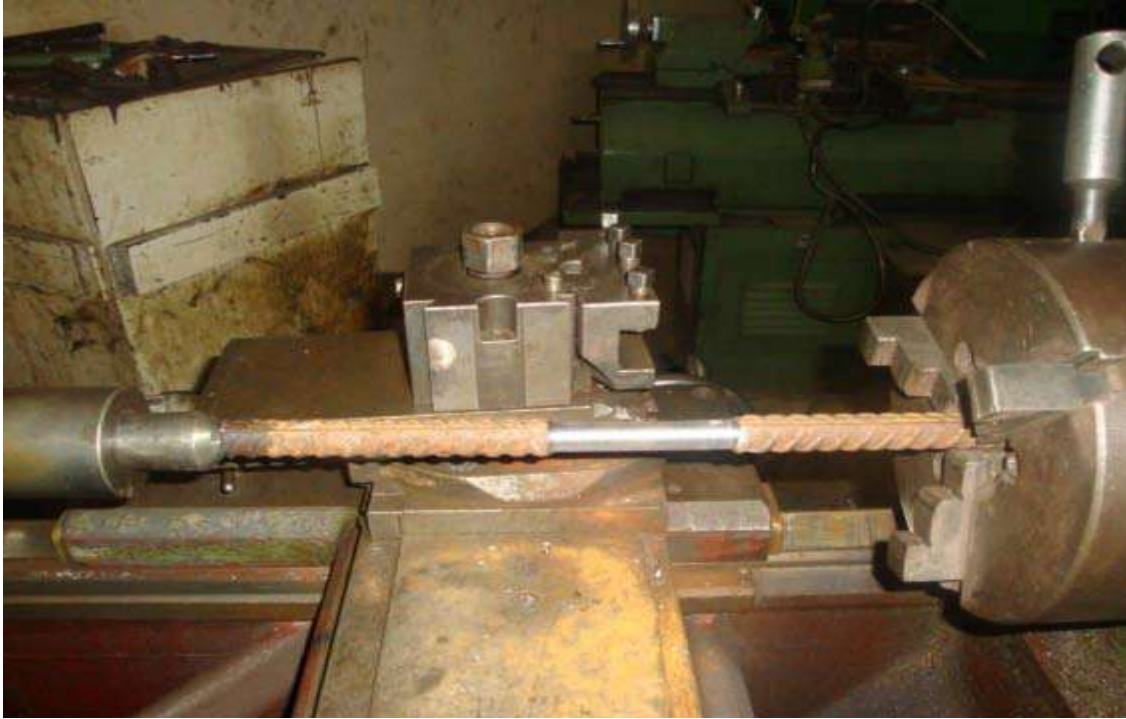
Plate 3.4: Sample test specimens being Machined using the Lathe Machine
