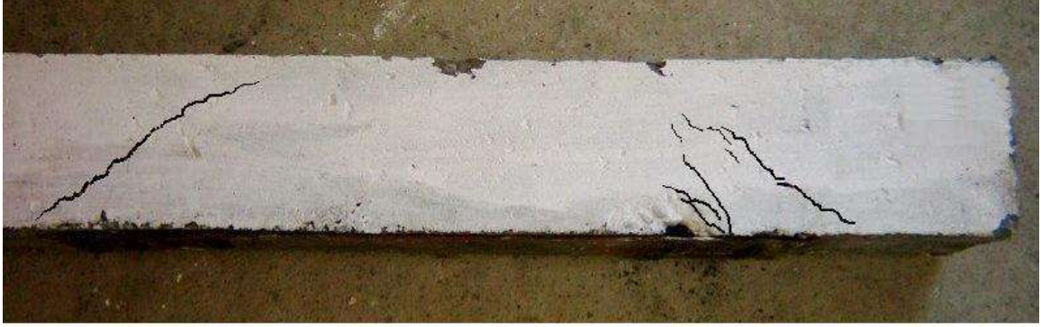
Plate 4.3: Crack Pattern at section of beam at ultimate stage of loading
