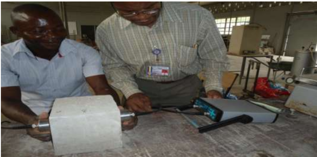
Plate 3.1: Determination of modulus of elasticity of concrete, E_c , by the U.P.V method
