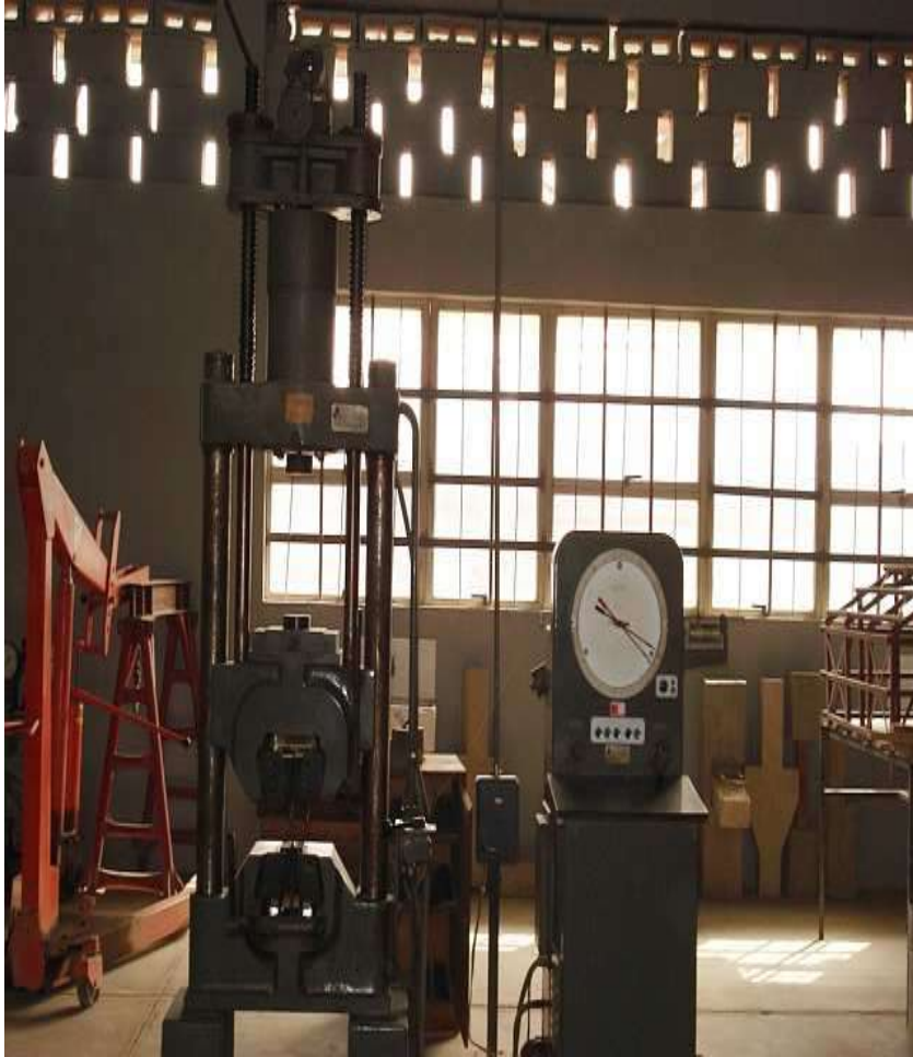
Plate 3.2: Universal testing machine used for the study
