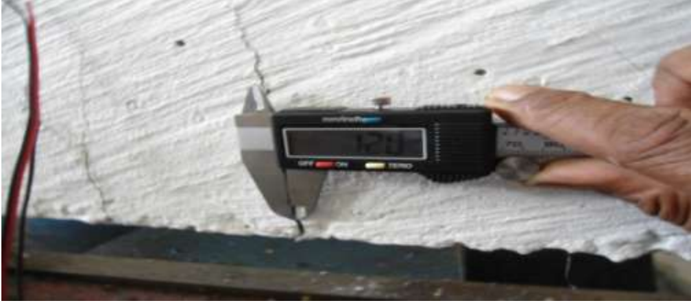
Plate 4.5: Measurement of crack width with digital Vernier Caliper.
