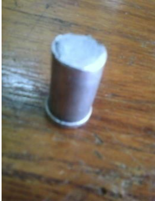
Plate 4.1: Aluminium alloy extruded with lubricant.
