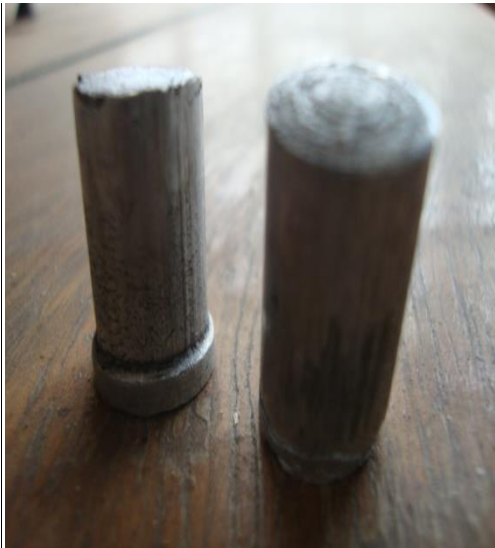
Plate 4.2: Aluminium alloy specimens extruded at 160 °C temperature without a lubricant
