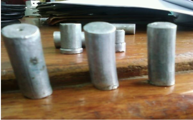
Plate 4.3: Extruded Aluminium specimens showing defects.
