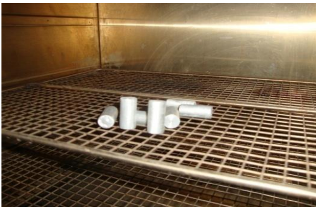
Plate 4.4: Aluminum alloy specimen being heated in an oven.
