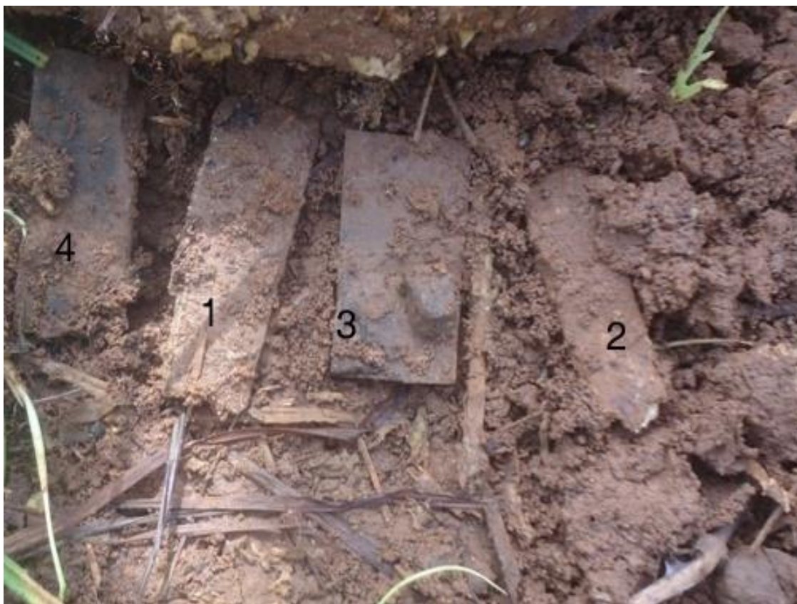
Figure.4.1: Residual of the wood samples after termite attack
