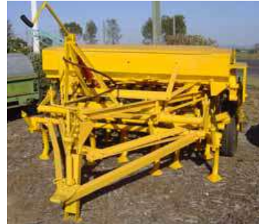
Plate 2.2: Drill planter (Murray et al. , 2006)
