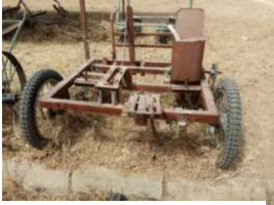
Plate 2.8. Two rows engine propelled seed ridge planter (Upahi 2017)
