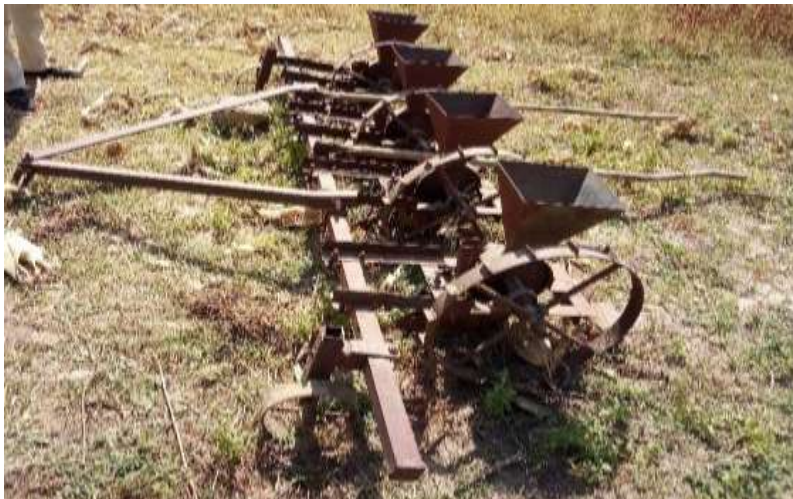
Plate 4.1. Planter diagram on the field
