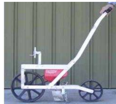
Plate 2.4: Precision planter (Murray et al. , 2006)
