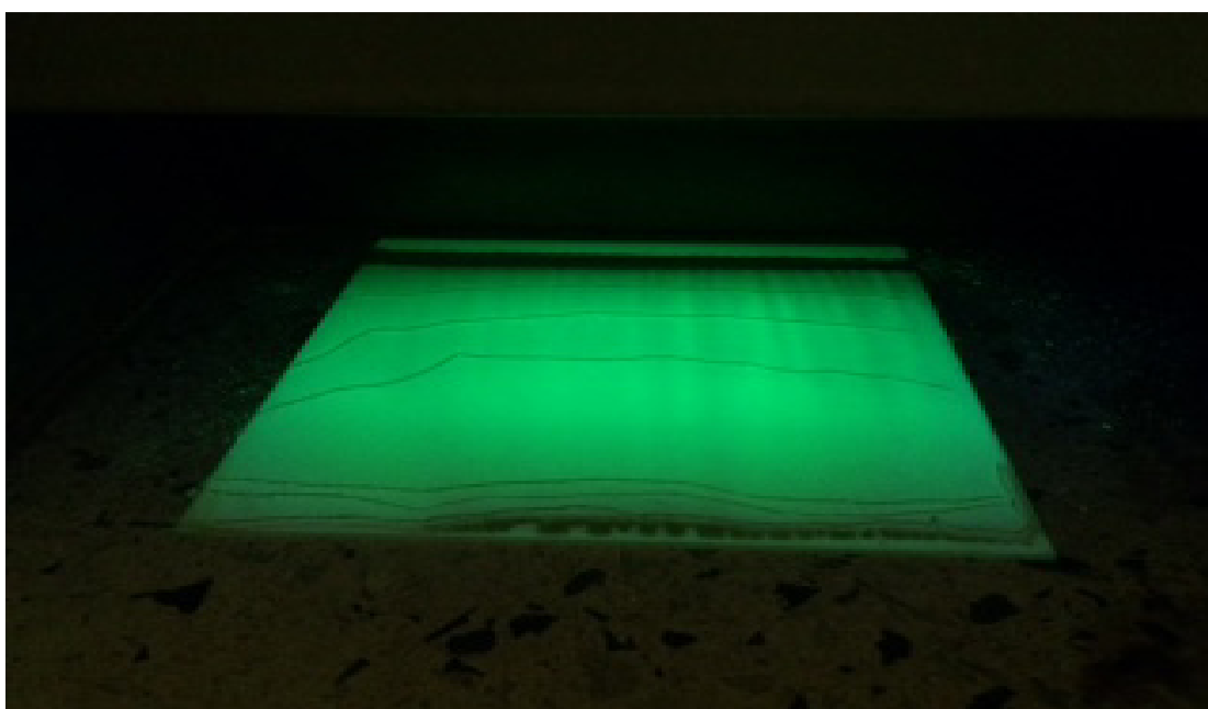
Figure 13 Picture of preparative TLC plate at UV 254nm of Compound AA-01
