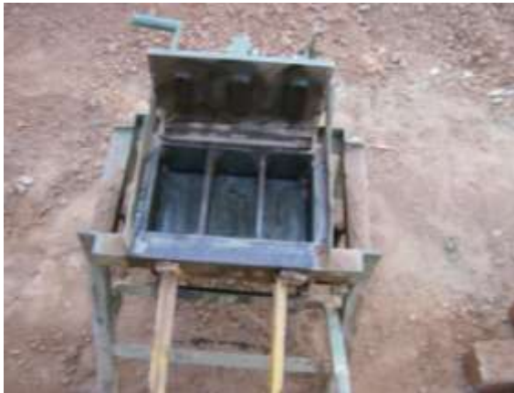
Plate3.1: Rammed Earth Blocks Mould
