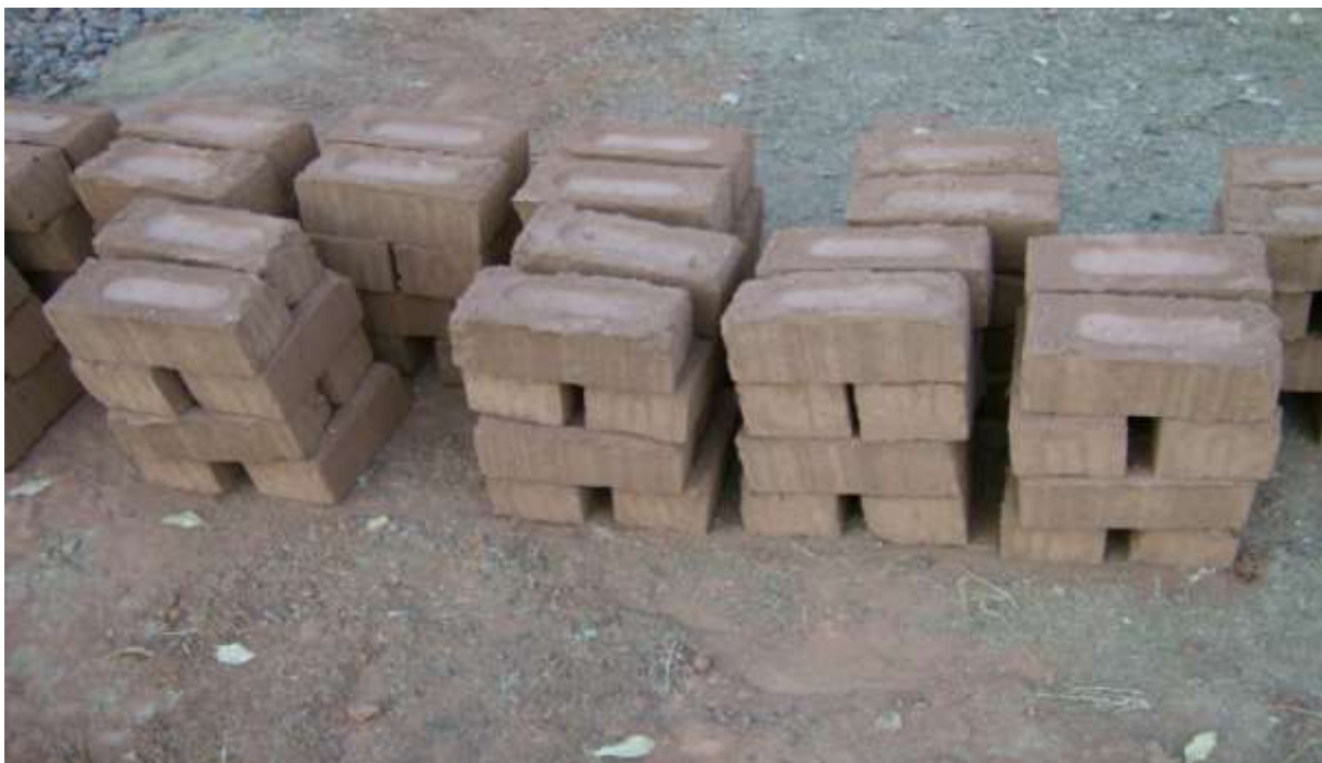
Plate 3. 3: Samples of produced stabilized laterite blocks
