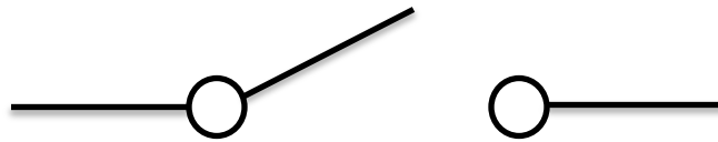
Figure 1.5 Circuit Symbol of a switch
