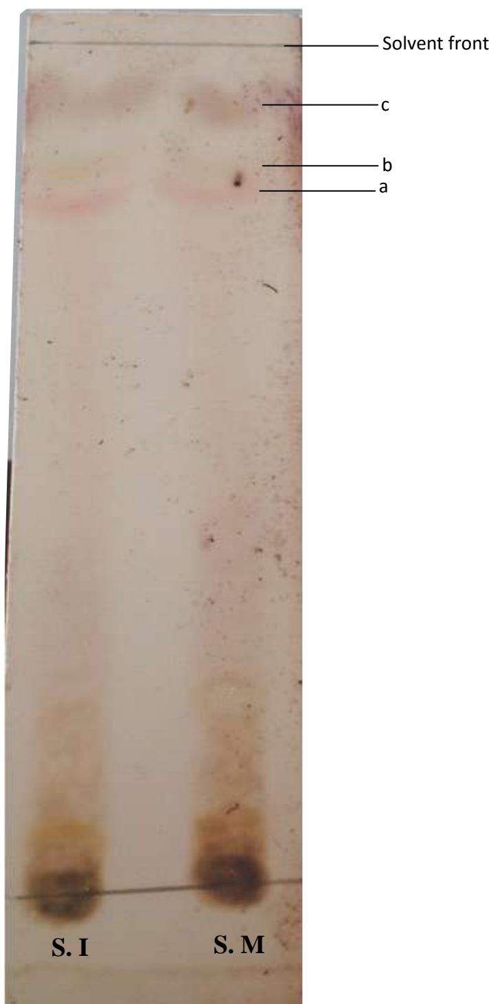
Plate XVII: Chromatogram of S. incanum and S. melongena developed in Chloroform (100%) and sprayed with Liberman-Burchard's reagent.
