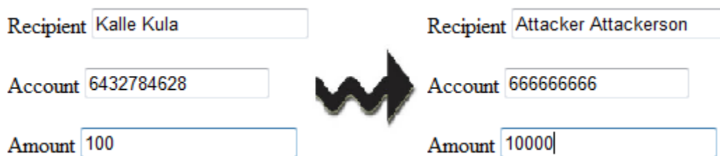
Figure 2.1: Example of a transaction altered during man in the browser attack(Nilsson, 2012). What makes MitB attacks difficult to detect from the bank's server side is that any activity performed seems as though it is originating from the legitimate user's web browser. Characteristics such as the Windows language and the IP address will appear the same as the user's real data. This creates a challenge in distinguishing between genuine and malicious transactions (RSA Lab, 2011).
