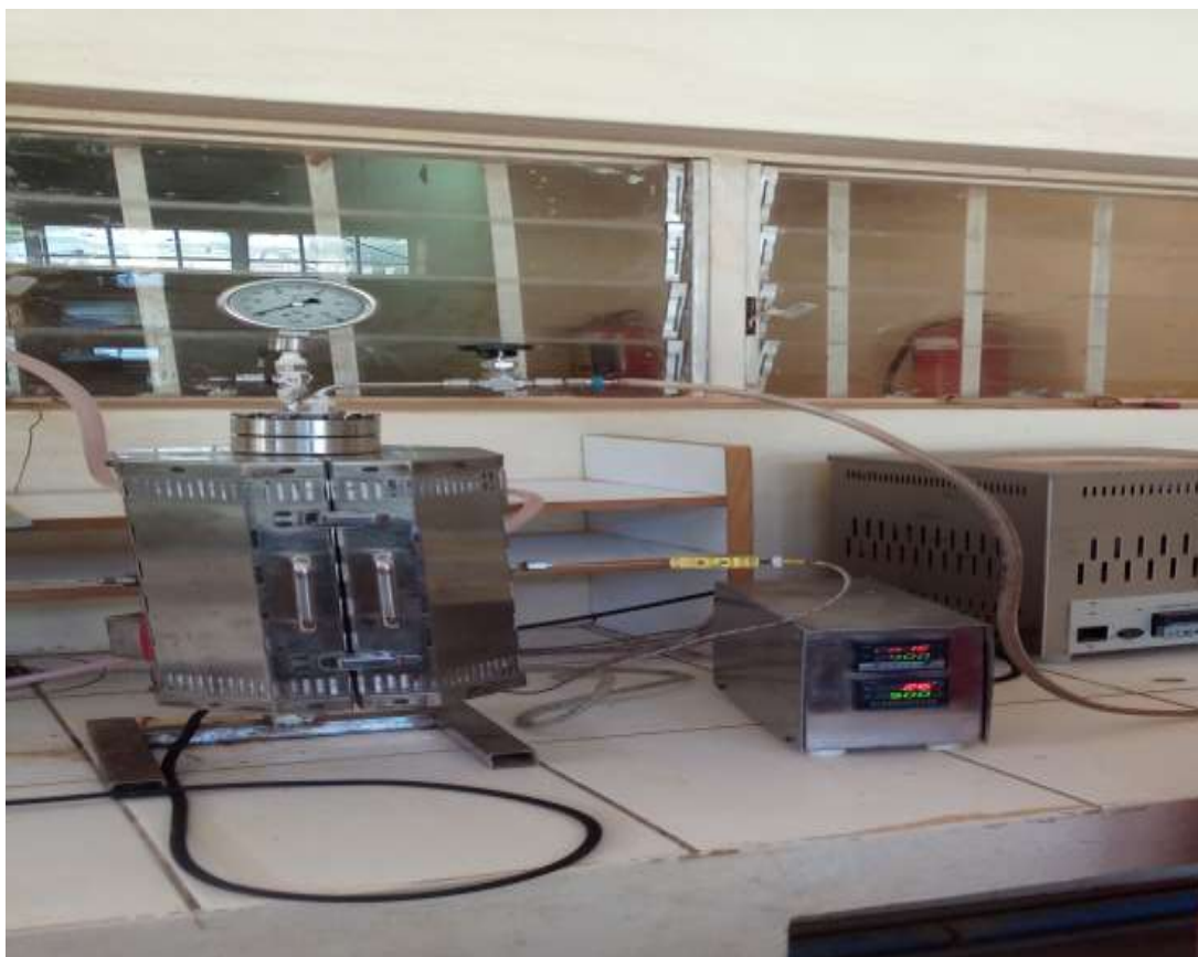
Plate 2.3 Setup Showing Hydrodeoxygenation Process
