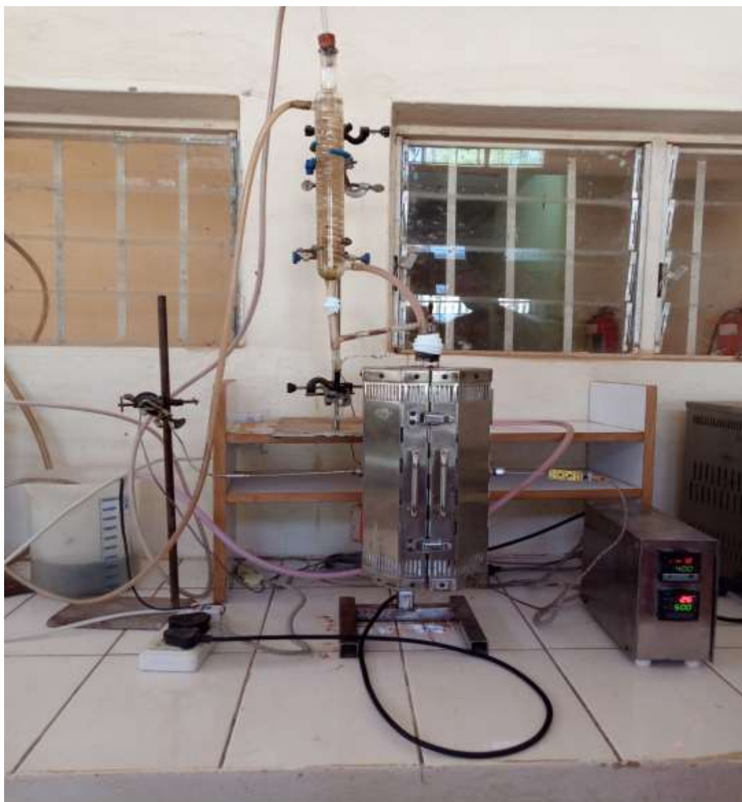
Plate 2.1 Setup Showing Furfural Production
