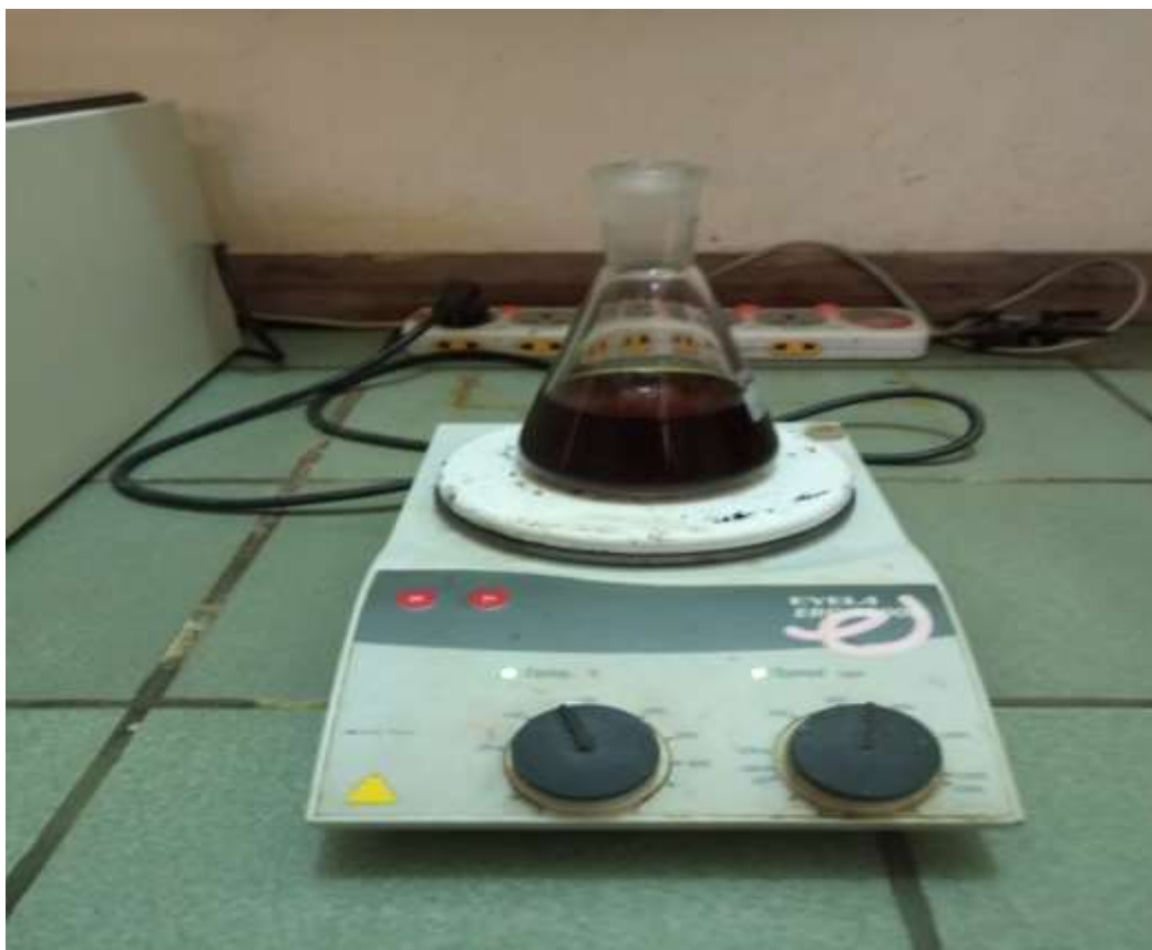
Plate 2.2: Setup Showing Condensation of Furfural with Acetone
