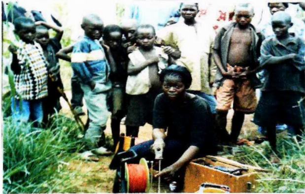
Figure 8: Driving electrodes into the ground during data acquisition
