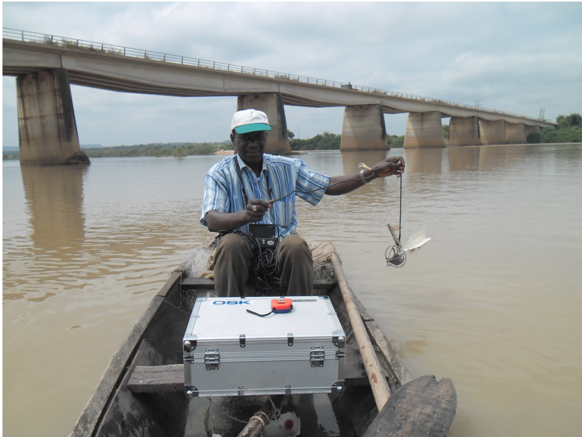
Plate 3: The shrinking river volume and measuring of discharge/velocity using current meter in Wuya Kpata Site3, During Dry Season
