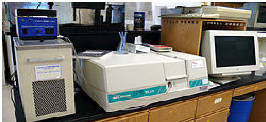
Plate. 3.2 Varian Cary 50Bio model uv 0906M012 uv-visible spectrophotometer (at Dept. Of Biochemistry B.U.K)
