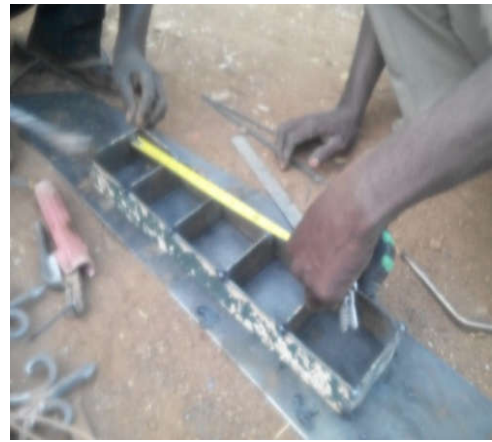
Plate III: Briquette moulders under construction
