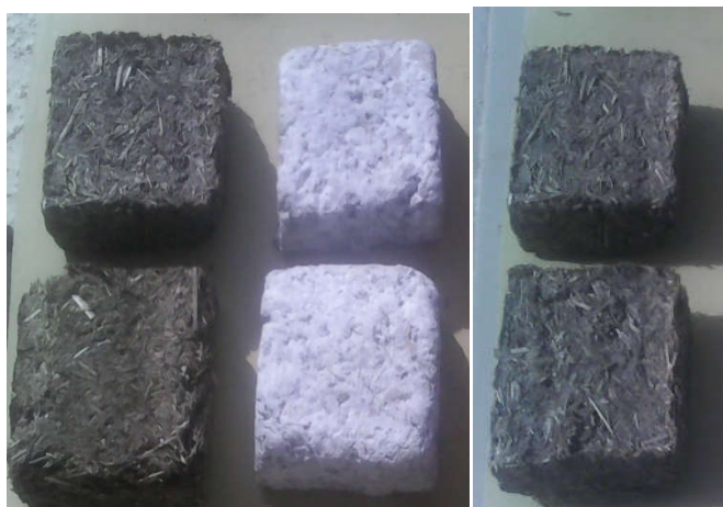
Plate X: Sun drying of the produced briquettes
