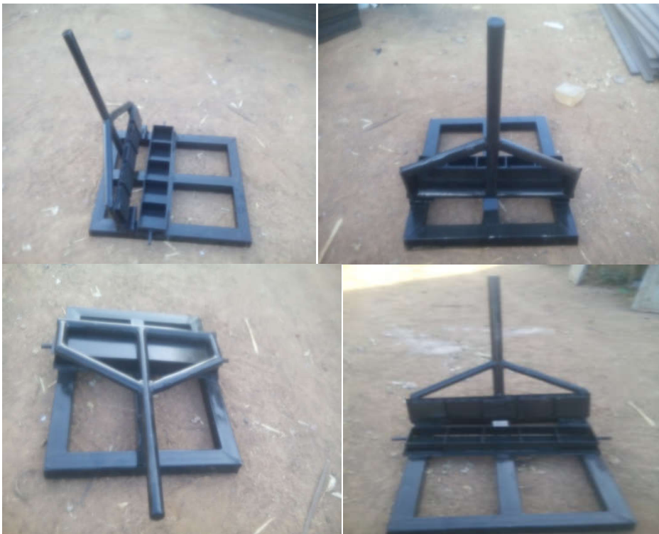
Plate V: Constructed Briquette moulder
