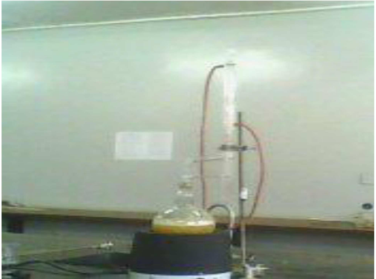
Plate iii: Modified Clevenger-type apparatus used for extraction of essential oils
