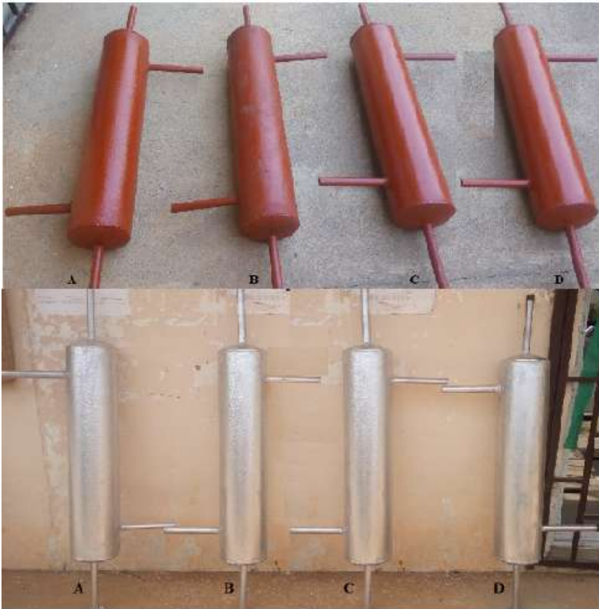
Plate 4.4: Images of Heat Exchangers (E-100 to E-103)
