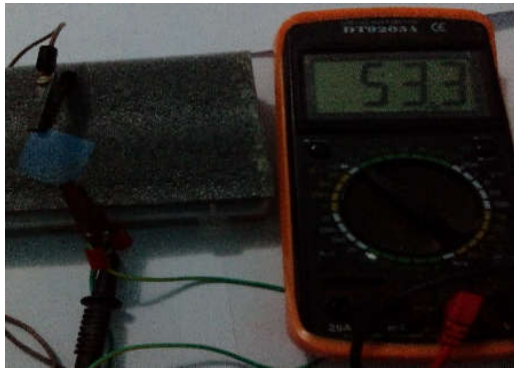
Plate 3: continuity test of conductive and non-conductive side of ITO glass slides
