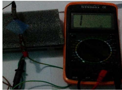
Plate 3: continuity test of conductive and non-conductive side of ITO glass slides
