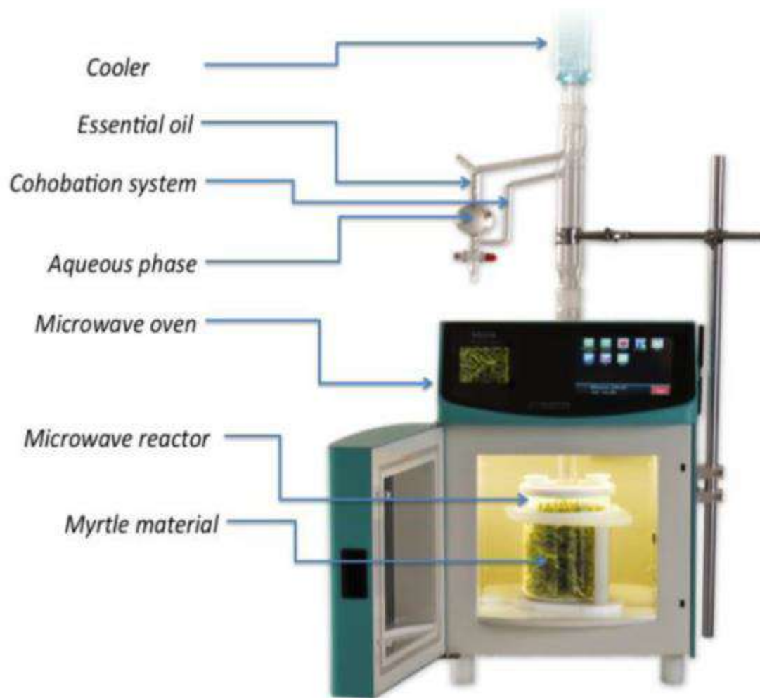
Fig 2.10: Solvent-free microwave extraction (Lucchesi et al. , 2007).
