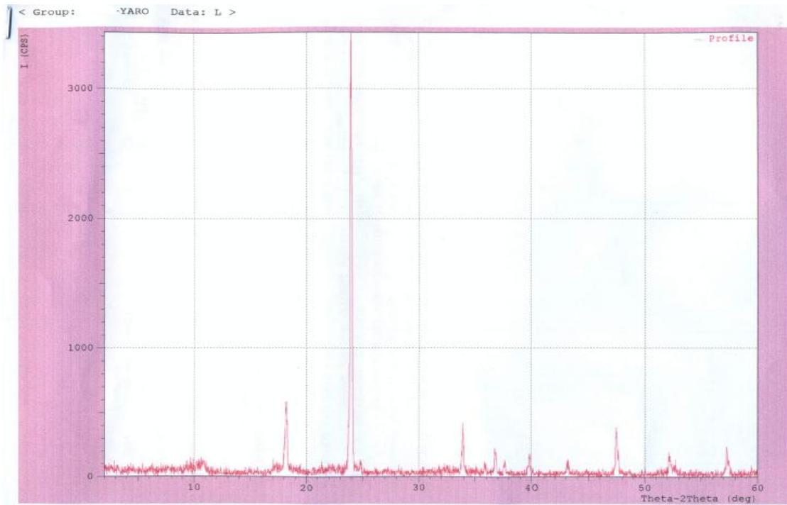
Figure 4.17: XRD patterns of glass-ceramics sample to which 4 wt% TiO<sub>2</sub> was added and then heat treated for 4 hours.
