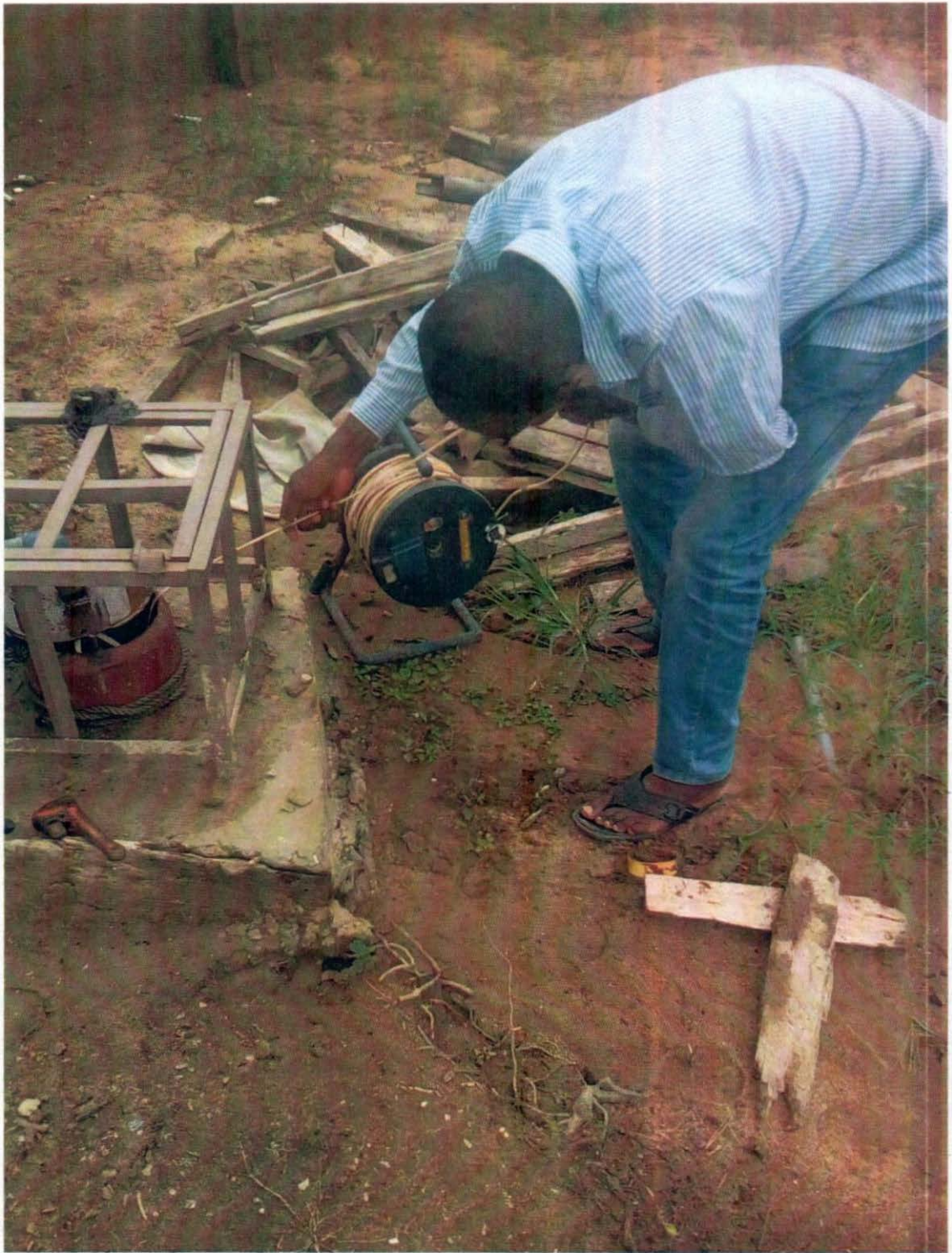
PLATE 2: Typical static water level measurement using water level probe at location 6BH (N 5° 1' 54.0", E 8° 22' 2.4")
