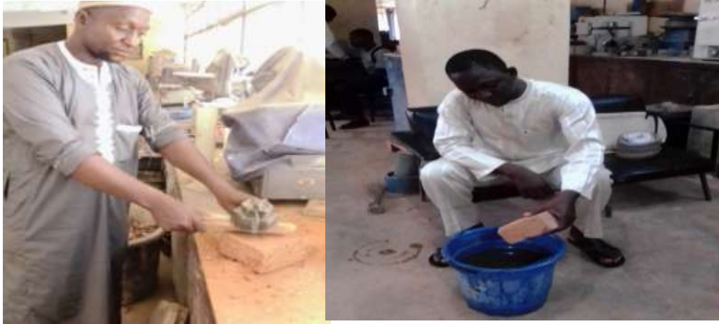
PLATE V: Abrasion resistance test
