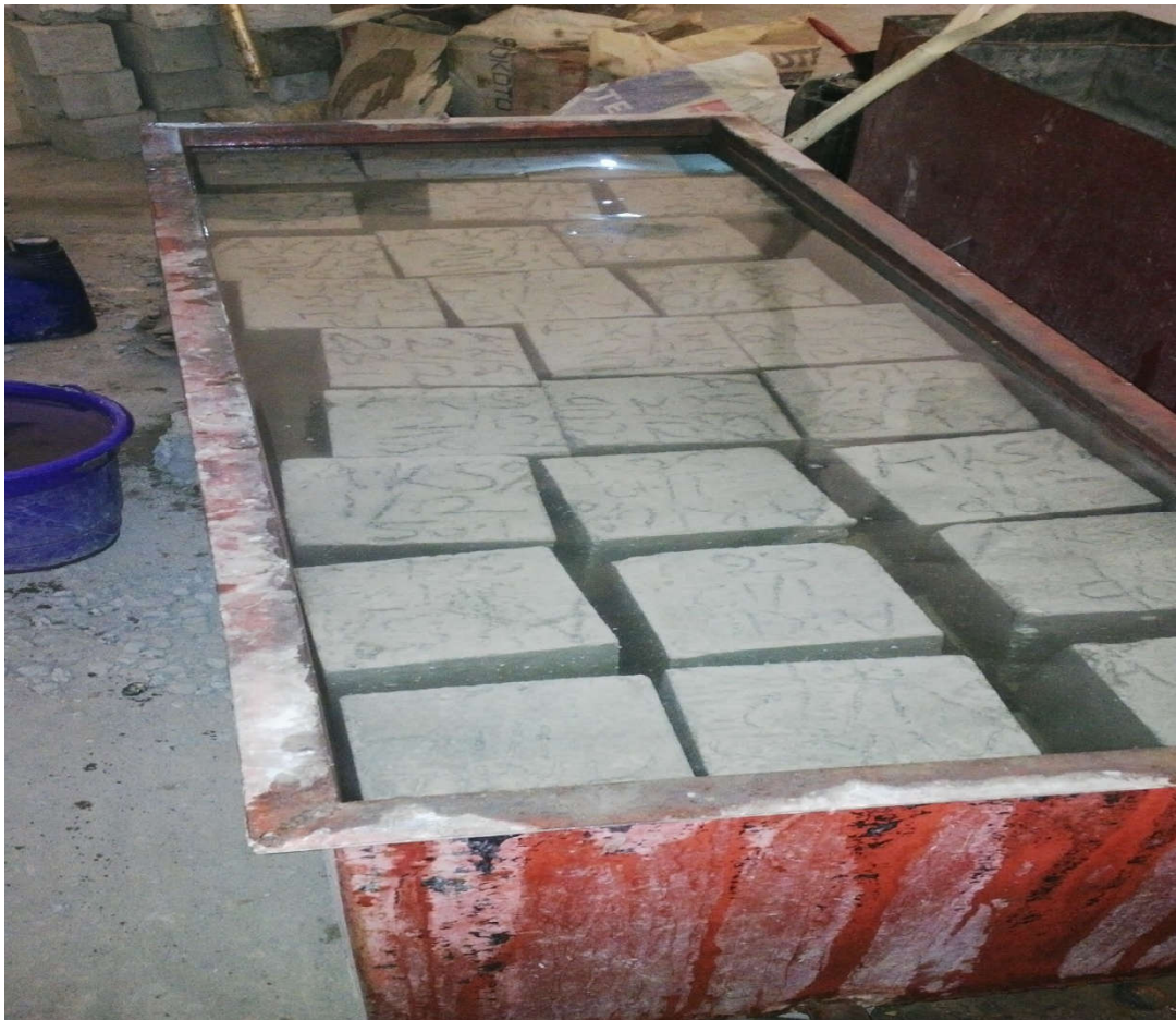
Plate II. Curing Of Concrete Cube in Water
