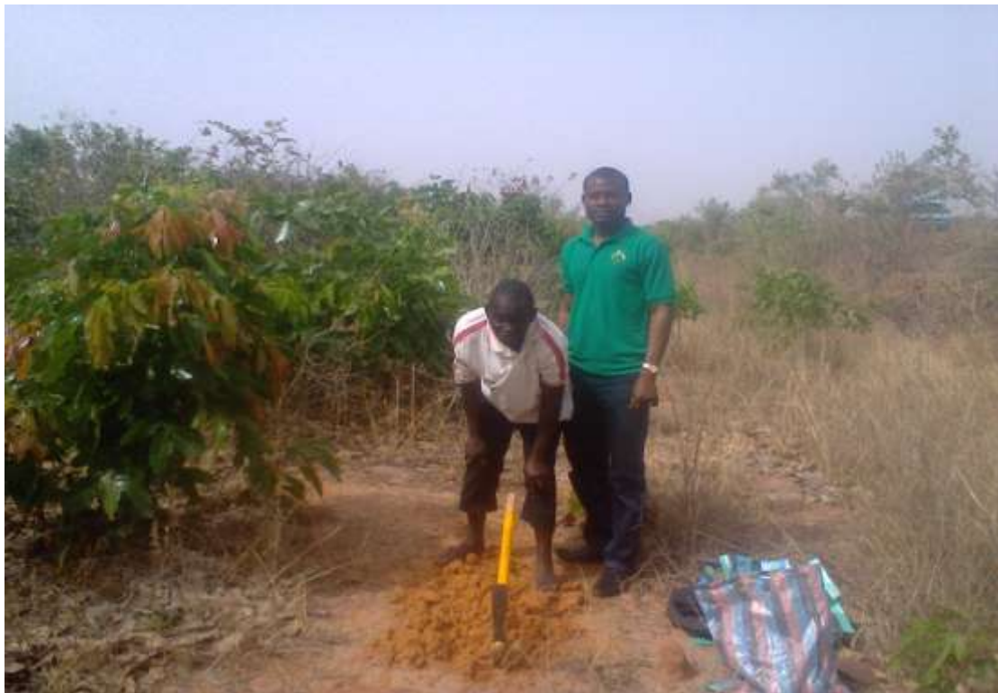
Plate III: The Researcher Obtaining Subgrade Soil Samples from MTS 1
