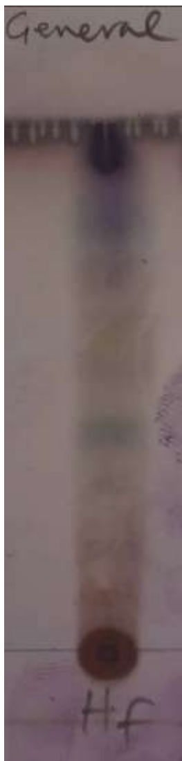
Figure 4.2: TLC Chromatogram of the extract sprayed with a general spraying reagent (P-anisaldehyde/H 2 SO 4 )
