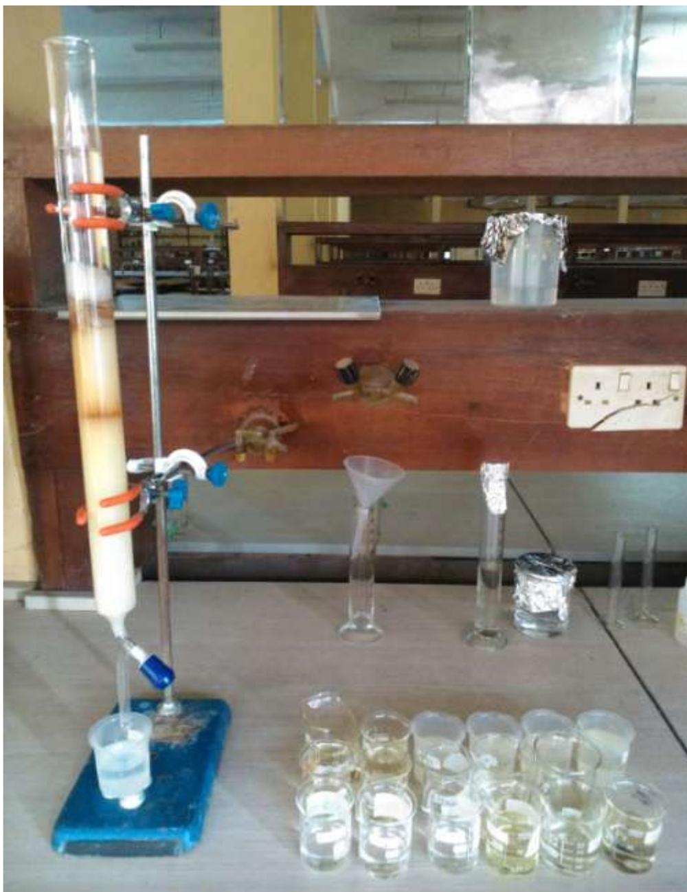
Set up for separation of *V. doniana* and *F. apodanthera* extracts using Column chromatography
