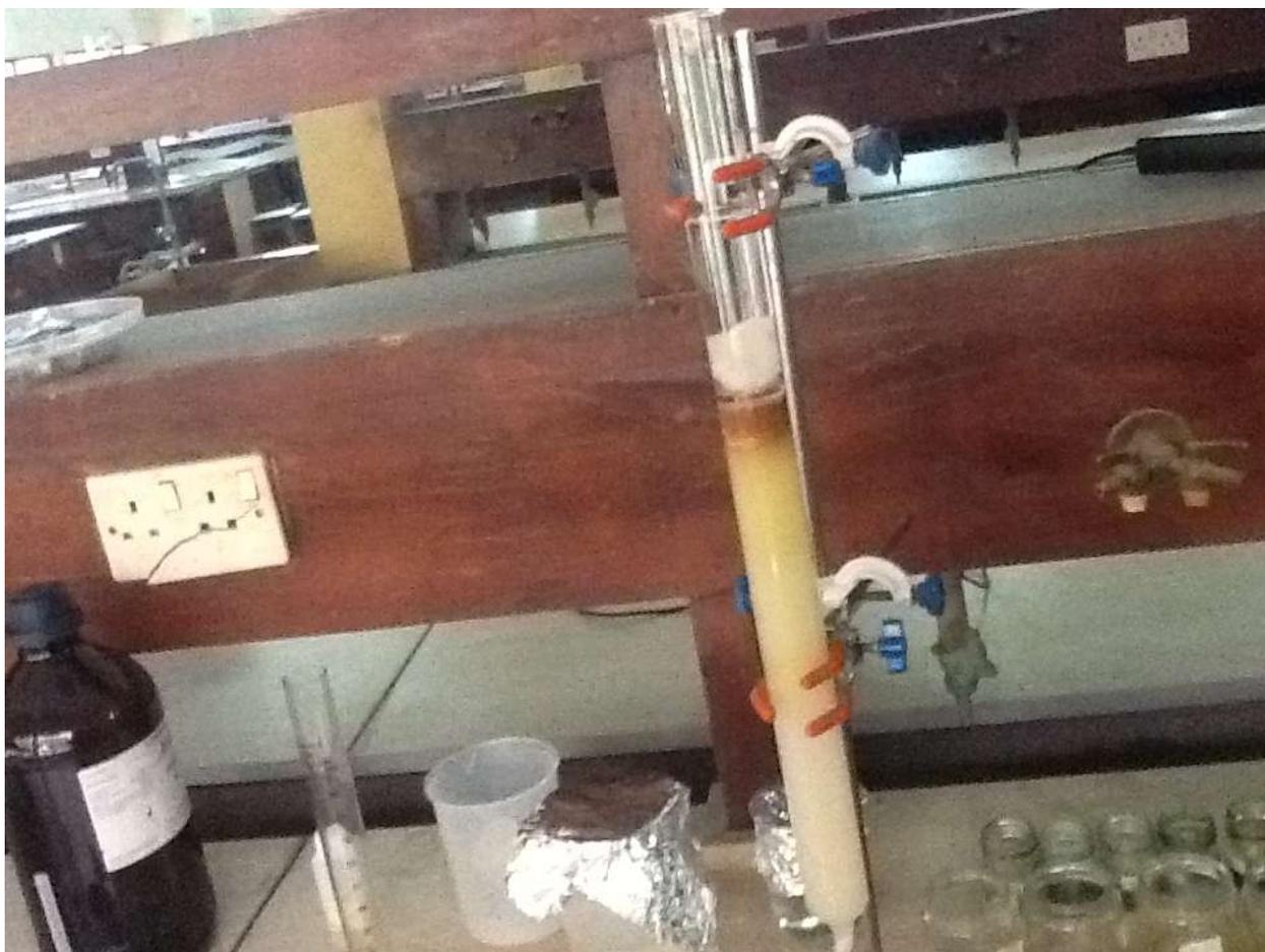
**Setup for column chromatography separation**
