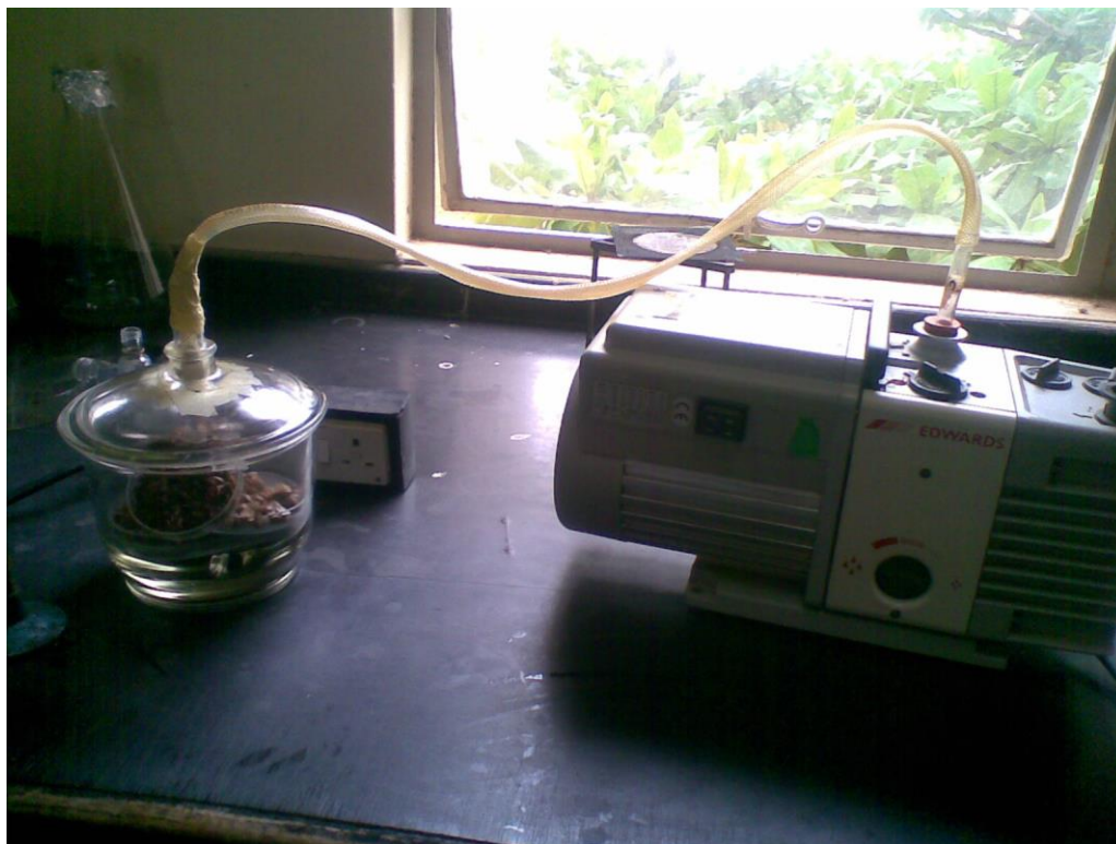
Drying of fermented P.africana , P.biglobosa and G.max seeds using a vacuum pump.
