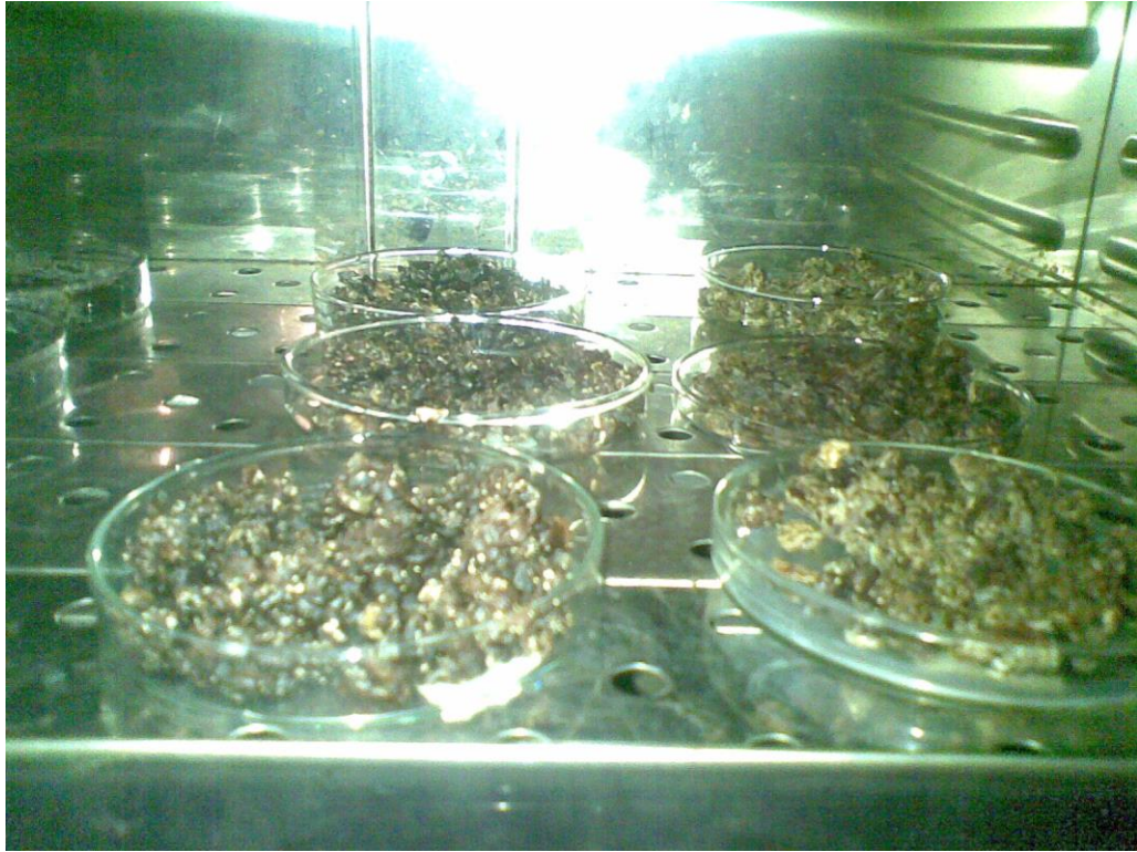
Drying of fermented P.africana , P.biglobosa and G.max seeds using hot air oven
