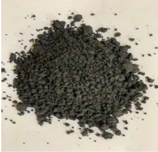
Figure 3.8: Mixture of Alawa Graphite & Clay for HB Pencil grade.
