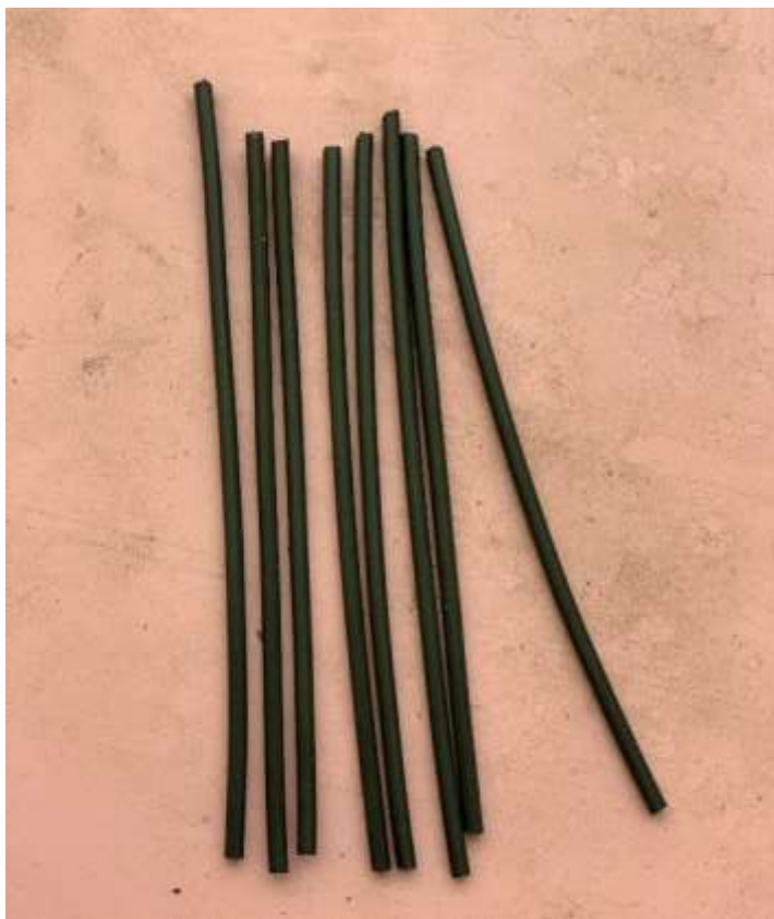
Figure 3.11: HB grade Pencil Leads made from Alawa graphite
