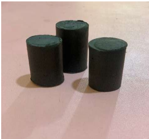
Figure 3.9: Cylindrical blocks produced from Alawa Graphite & Clay mixture for HB pencil grade
