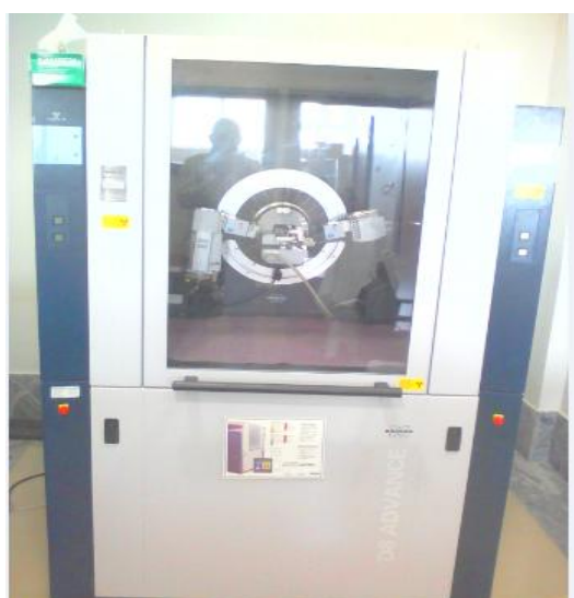
Plate 3.12: XRD machine (African Development Bank Laboratory, African University of Science and Technology, Abuja)
