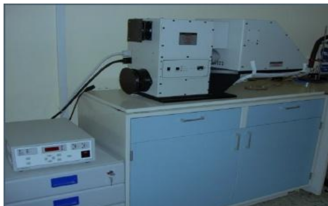
Plate 3.13: Solar simulator (African Development Bank Laboratory, African University of Science and Technology, Abuja)
