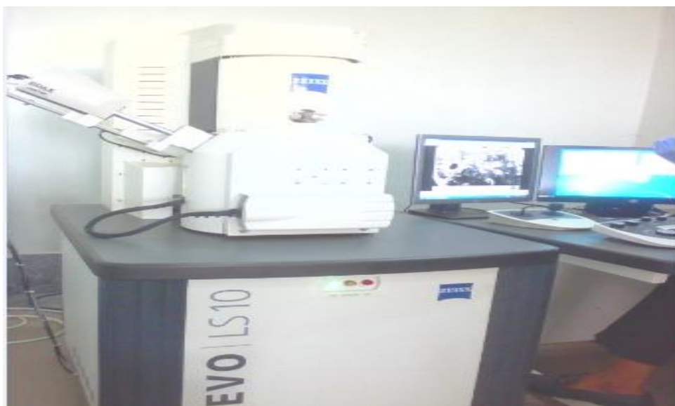
Plate 3.9: Scanning Electron Microscope (SEM) with EDS (African Development Bank Laboratory, African University of Science and Technology, Abuja)
