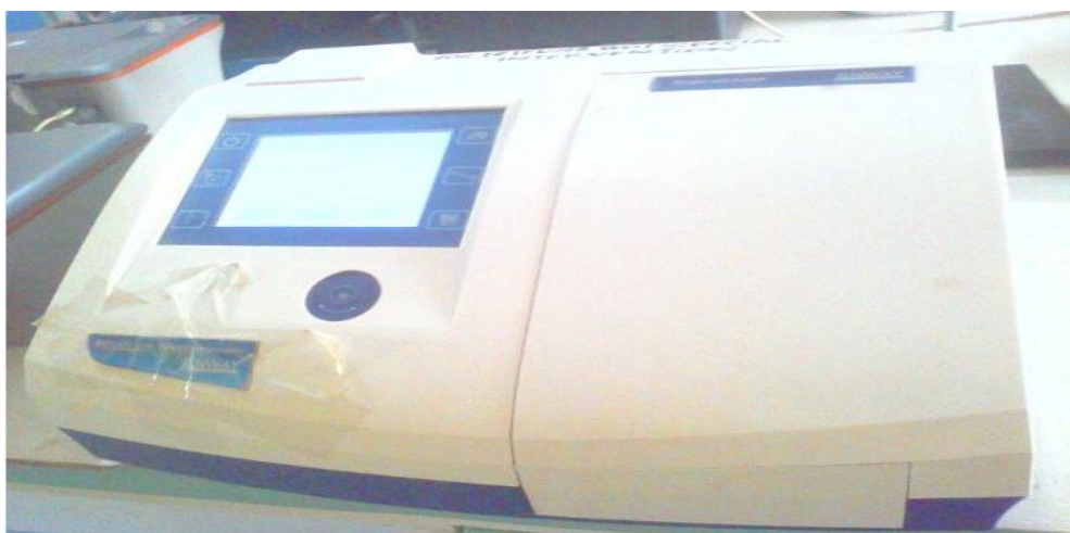
Plate 3.10: UV-VIS Spectrophotometer (Materials Science and Engineering Laboratory, Kwara State University, Malete)
